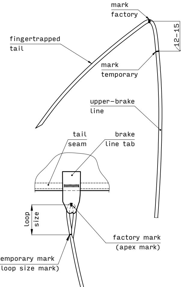
Before attaching the lines to the tail, mark all the upper brake lines with small temporary marks at your desired loop size. We suggest:
