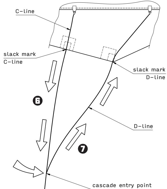
Once identified, pull the lines slightly to ensure they remain even and straight. Next, place a mark on the D-line **8**, 15 mm towards the canopy from the position of the mark on the C-line.
